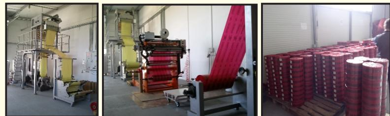
Attention tapes are made of a single layer PE film on which is, depending on the type of installation to where is applied, warning clearly written. For example, warning – power cable, telecom cable,...Also, depending on the type, it is made in red or yellow or in the colour the customer requests. All tapes are rolled on a paper tube, marked with labels and packed in a protective film. Standard weight of a colis is 4 to 8 kg.
